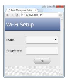
After a click on the OK button the Light-Manager starts connecting to the selcted Wi-Fi network. During this phase the LED is blinking in green. When this is done the LED stops blinking and changes its color to dim blue to signal operational readiness. Now the Light-Manager is connected to your Wi-Fi network and the IP address is shown in AirStudio under options -> Light-Manager setup. This setting can be changed in the options, too.
